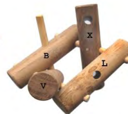
SECOND STEP, MAKE TWO OF THESE SUBASSEMBLIES
